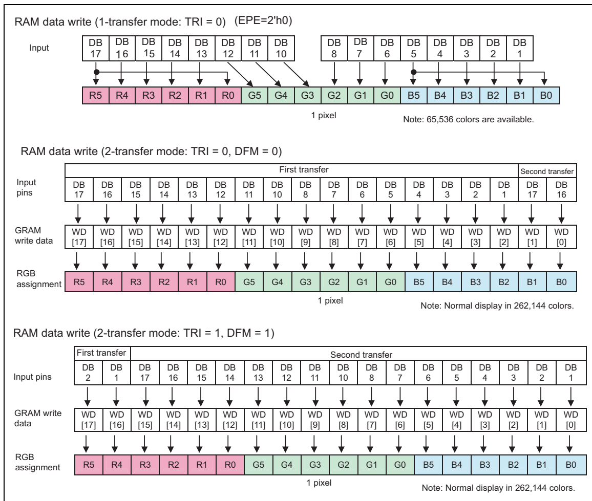
Figure 19 16-bit Interface Data Format (RAM Data Write)
